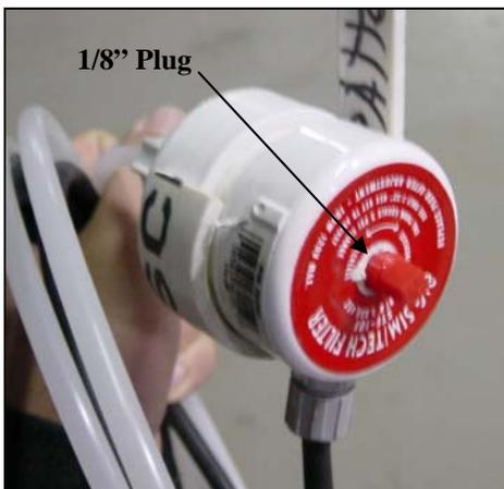
1. Remove 1/8" plug on top of switch and insert 7/32" hex wrench.
